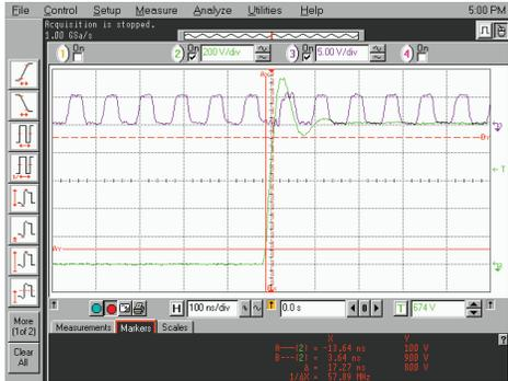
$dV/dt = 45 \text{ kV}/\mu\text{s}$
