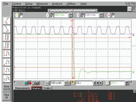
$dV/dt = 45 \text{ kV}/\mu\text{s}$
