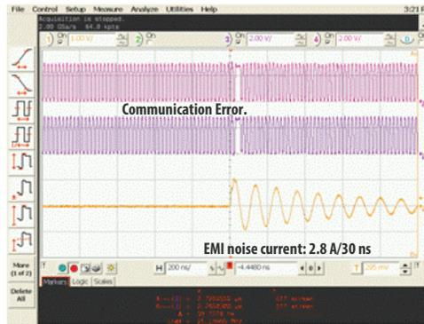
Magnetic Isolator – Missing bits seen at 2.8 A of loop current nearby.
