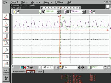
$dV/dt = 45 \text{ kV}/\mu\text{s}$
