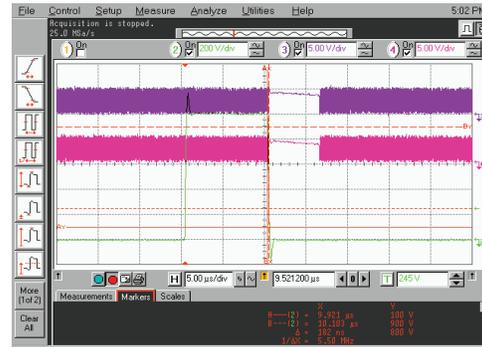
$dV/dt = 4 \text{ kV}/\mu\text{s}$
