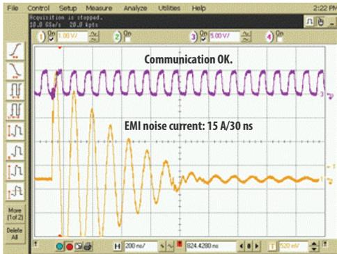
Broadcom Optocoupler – No missing bits seen at 15 A of loop current nearby.
