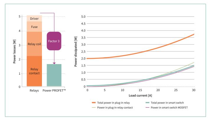
Figure 2: PROFET<sup>™</sup> devices offer a significant drop in power dissipation compared to the plug-in relays they replace.
