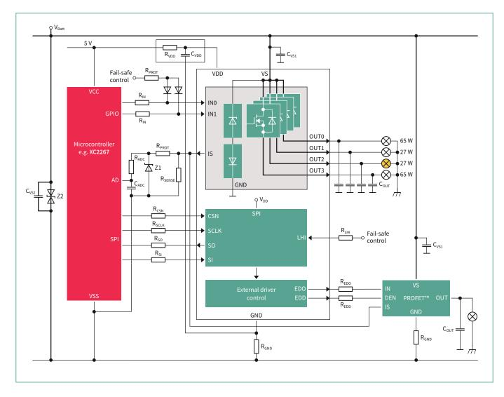
Figure 5: SPOC<sup>™</sup> +2 multi-channel high-side switches provide both control and diagnostic capability via SPI.
