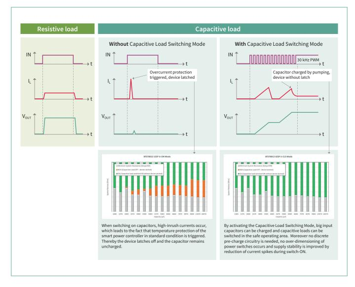
Figure 4: The newly released PROFET<sup>™</sup> +2 12V products BTS70012-1ESP, BTS70015-1ESP & BTS70020-1ESP are equipped with the latest feature, called **Capacitive Load Switching Mode**
