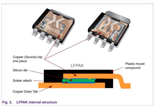
This section briefly discusses the main components in the internal structure of LFPAK MOSFETs and their temperature properties:
