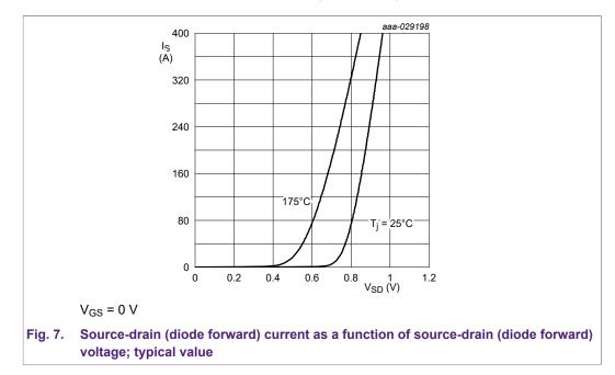
The above graph is obtained by testing the device with pulsed current to avoid self-heating, (which would result in higher values for  $V_{SD}$ ). In real applications self-heating will most likely occur, as currents lasting more than 100 ms will be sufficient to get  $R_{th}$  in steady state region and allow the device to heat up.
