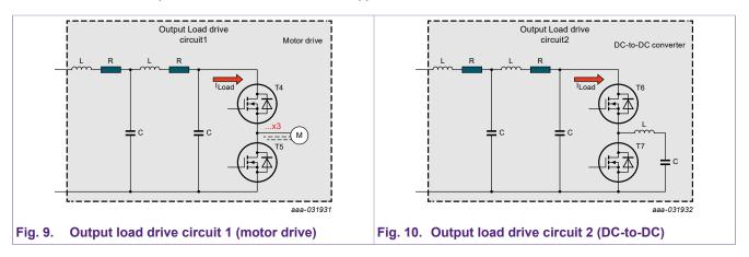
In this example we look at output load drive circuit 1, T4 and T5 in relation to current demand which will be gated by the type of motors driven and the power requirement of the application.
