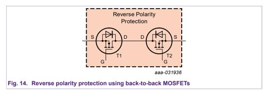
In a back-to-back configuration the other parameter that becomes of relevance is the avalanche performance of the MOSFETs. A situation where a fault condition occurs and T2 turns off as part of a protection mechanism. Due to inductances in the cable and/or the circuit a build-up of a voltage at the drain of T2 might occur and potentially lead to an avalanche event. For details on avalanche topic see NEXPERIA application note *AN10273*.
