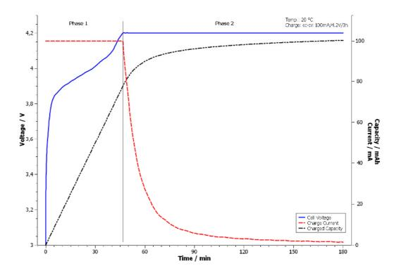
Figure 1. illustrates the different phases during a rapid charge cycle.
