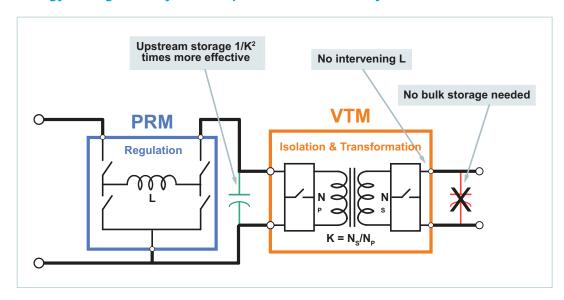
For faster load transient response that is often required in demanding applications such as radar and ATE test heads, the SAC<sup>TM</sup> topology by virtue of employing a fixed-ratio converter has the advantage of not imposing the bandwidth limitations of an internal control loop struggling to maintain regulation. Thus, the VTM<sup>TM</sup> powertrain offers a unique capacitance-multiplication feature.
