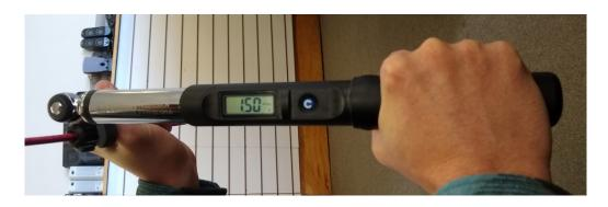
4.4.4 Tighten BOTH Sealing Caps completely by hand or to the following torque specifications. Or using wrench tool AMPVTW0001 to tighten the two Sealing Caps.
