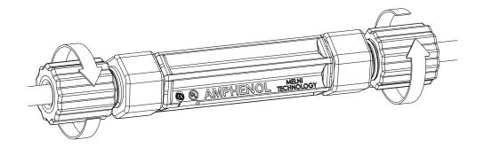
4.4.3. Using a Calibrated Torque Wrench and either a 3/4" or 20mm crows foot adapter, tighten BOTH of the Racheting End Capts to the EXACT specified torque shown in the table below. Or using wrench tool AMPVTW0001 to tighten the two Racheting End Caps.
