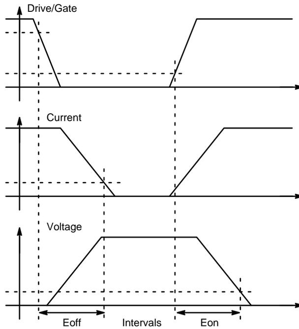
**Figure 26. Turn-On and Turn-Off Energy Measurement**
