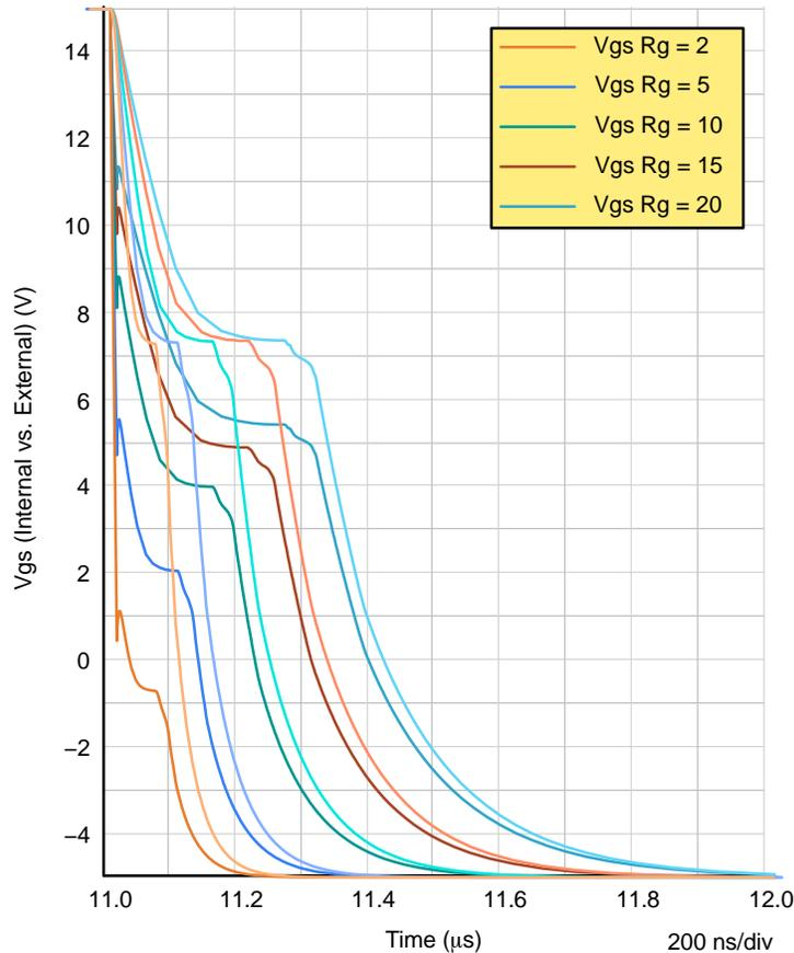
**Figure 9. Gate-to-Source Voltage Difference between Internal and External with High Internal Gate Impedance**
