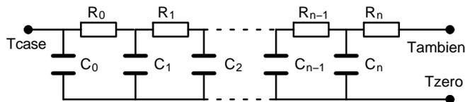
**Figure 21. Cauer Network for a 1-Inch Square PCB**
