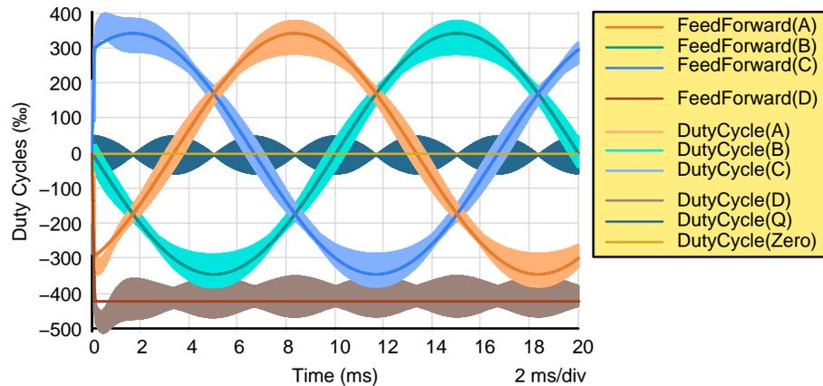
**Figure 41. Feed Forwards and Duty Cycles WITHOUT 3<sup>rd</sup> Harmonic Injection**
