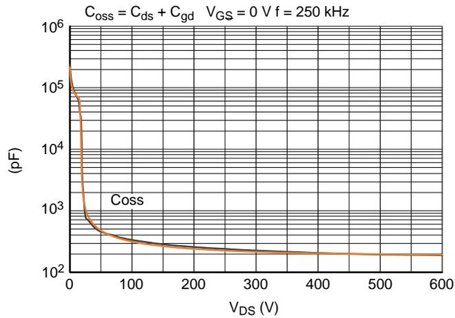
**Figure 2. Physical & Scalable Model Output Capacitor Simulation Results**
