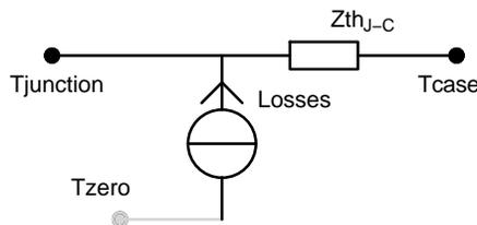
**Figure 18. Internal Thermo-Electrical Structure**
