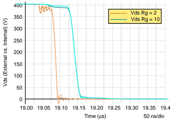
**Figure 6. Drain-to-Source Voltage Difference at Turn-On between Internal and External**
