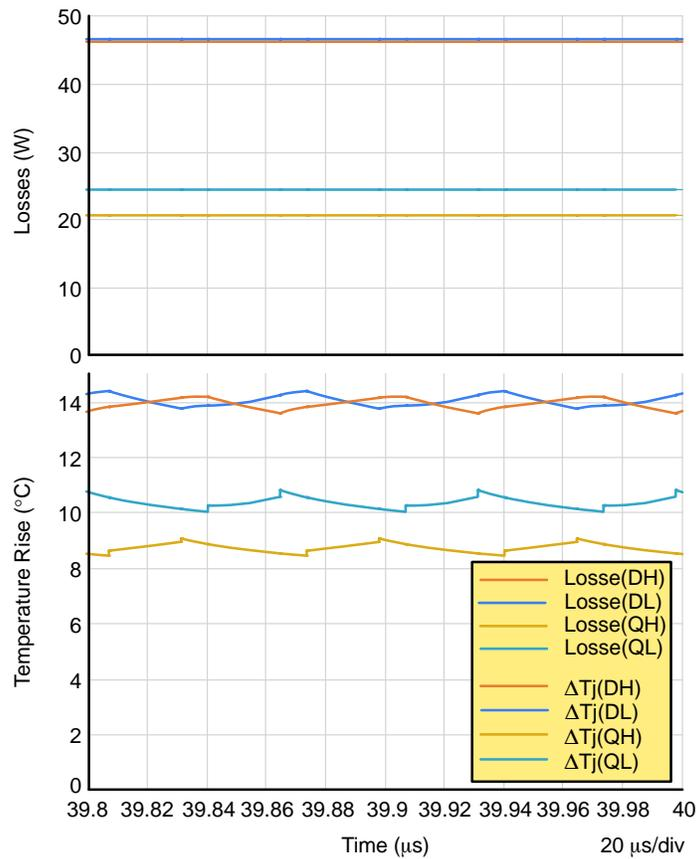
**Figure 35. Losses and Junction Temperature Rise with High External Gate Resistor**
