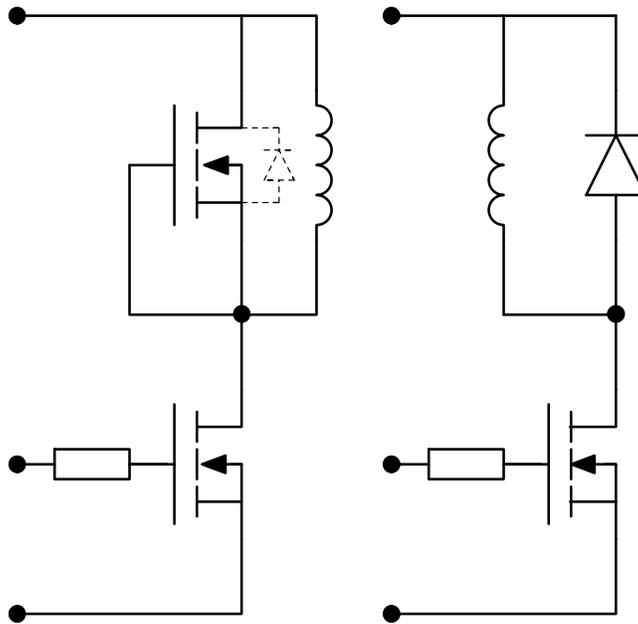
**Figure 27. Half-Bridge and Quarter-Bridge Structures**
