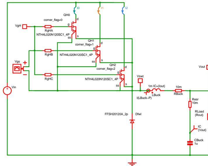
Figure 11. Buck Stage with Corner Models
