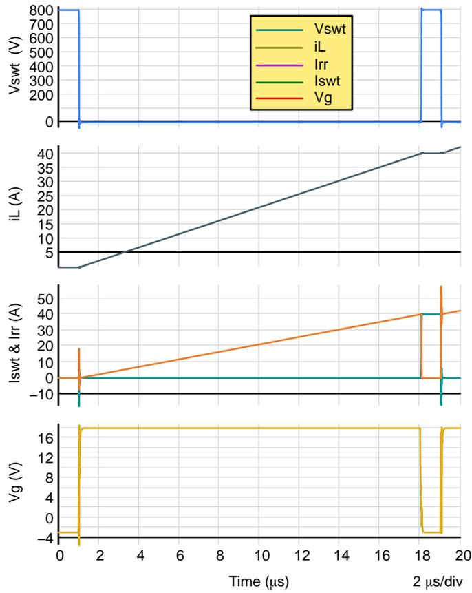
**Figure 25. Double Test Waveforms**
