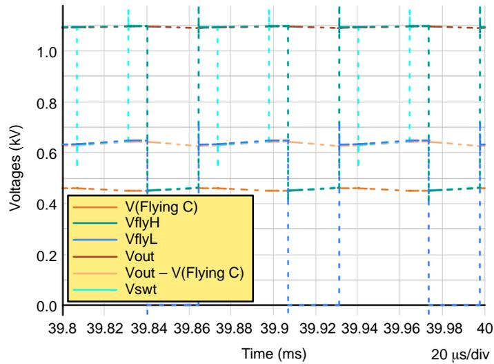
**Figure 31. Flying Capacitor Boost Capacitor Voltages Waveforms**
