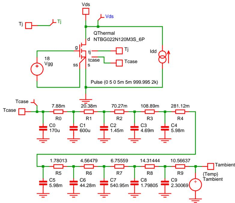
**Figure 22. Simulation Schematic with Cauer Network**
