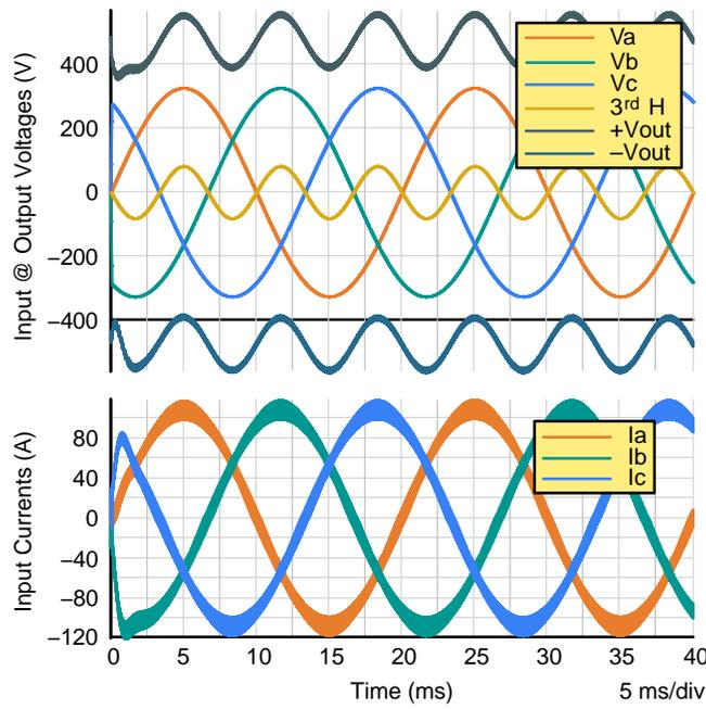
**Figure 39. Input and Output Waveforms WITH 3<sup>rd</sup> Harmonic Injection**
