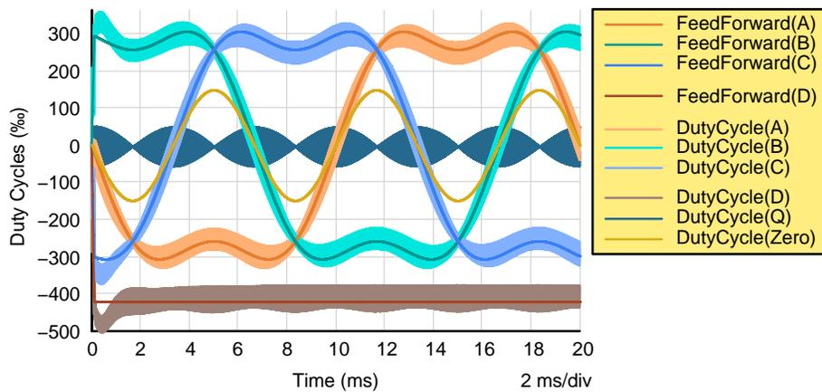
**Figure 42. Feed Forwards and Duty Cycles WITH 3<sup>rd</sup> Harmonic Injection**
