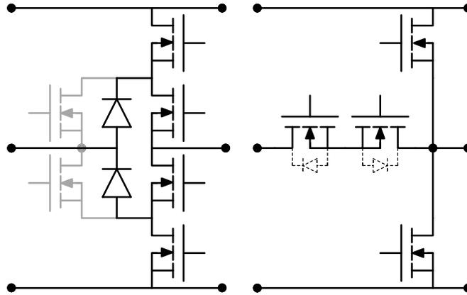
**Figure 36. I–NPC (A–NPC in Grey) and T–NPC Cells**
