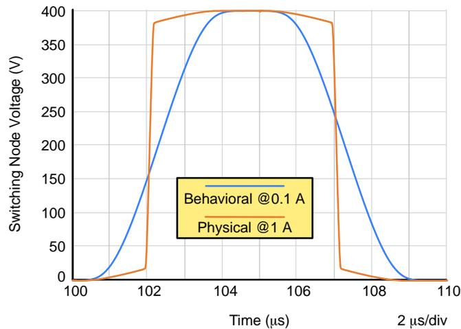
**Figure 4. Output Capacitor Simulation Results Comparison Behavioral vs. Physical and Scalable**
