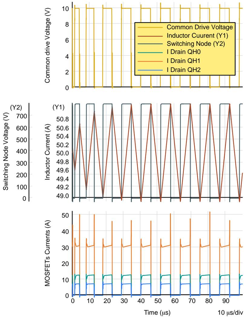
Figure 12. Buck Stage Waveforms with SiC MOSFET Corner Models
