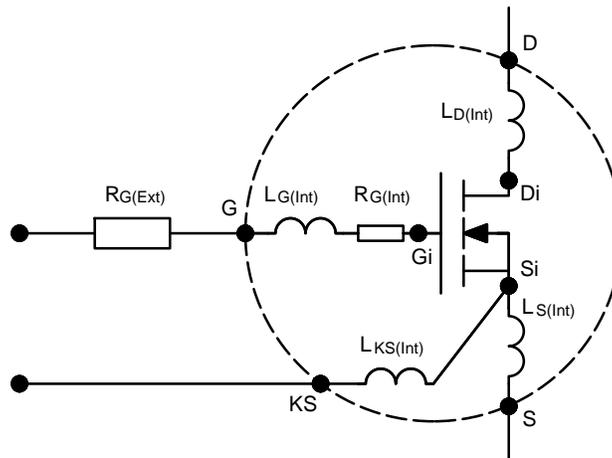
**Figure 5. Internal Versus External Nodes**
