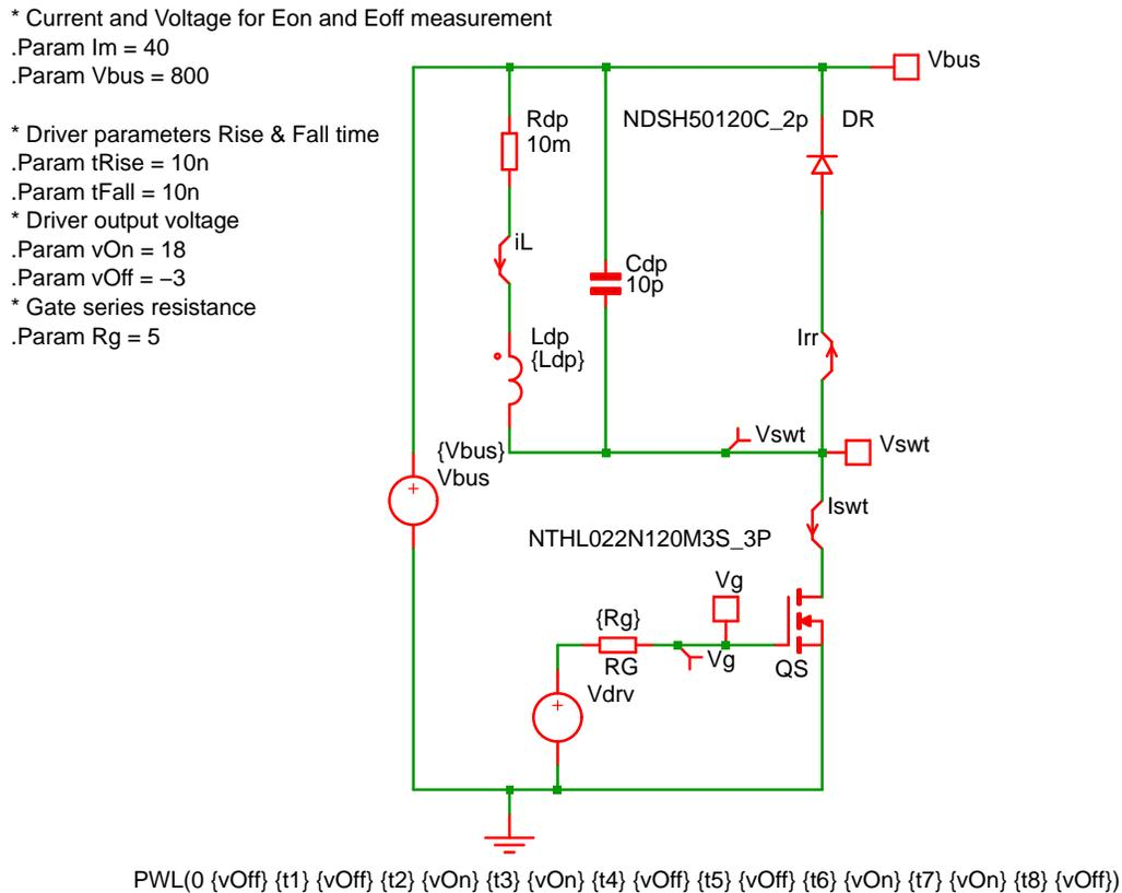
**Figure 24. Double Pulse Tester Simulation Schematic**
