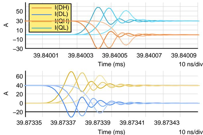
**Figure 34. Flying Capacitor Boost MOSFETs Turn-On Current Waveforms Zoom vs. External Gate Resistor**
