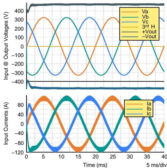
**Figure 38. Input and Output Waveforms WITHOUT 3<sup>rd</sup> Harmonic Injection**
