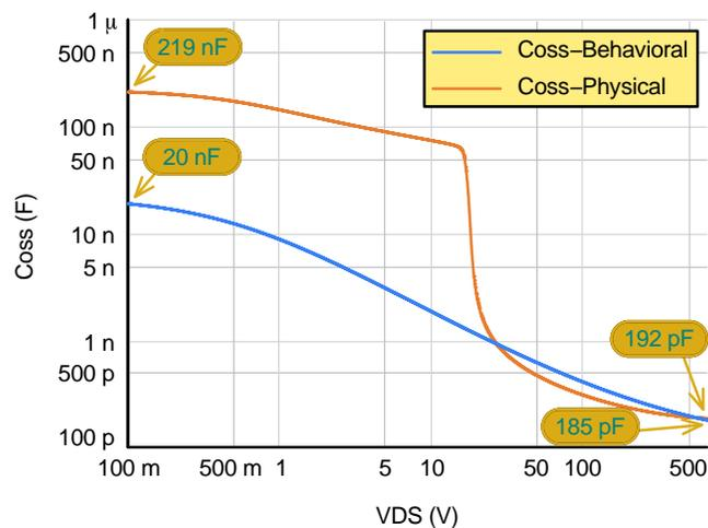
**Figure 3. Output Capacitor Simulation Results Comparison Behavioral vs. Physical and Scalable**
