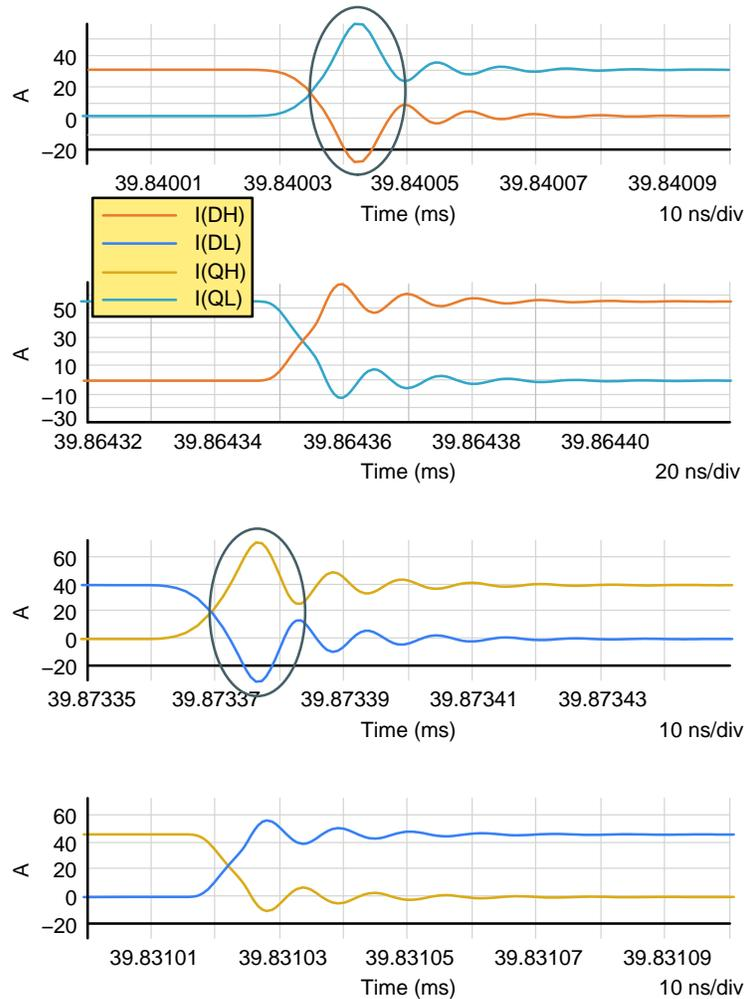
**Figure 32. Flying Capacitor Boost Switches Turn-On and Off Current Waveforms Zoom**
