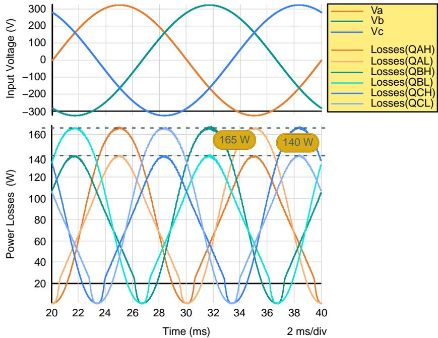
**Figure 44. Losses with Third Harmonic Injection Over On Grid Period**
