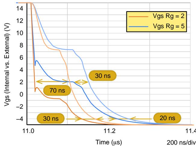
**Figure 10. Gate-to-Source Voltages Delays**
