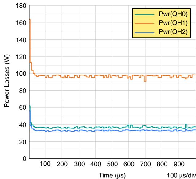
**Figure 16. Total Power Losses in Each SiC MOSFET**
