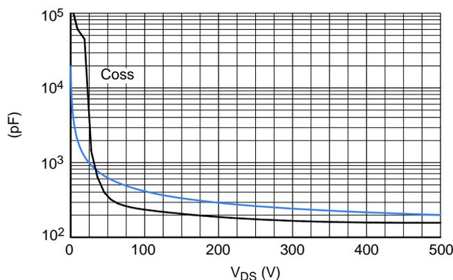
**Figure 1. Behavioral Model Output Capacitor Simulation Results**
