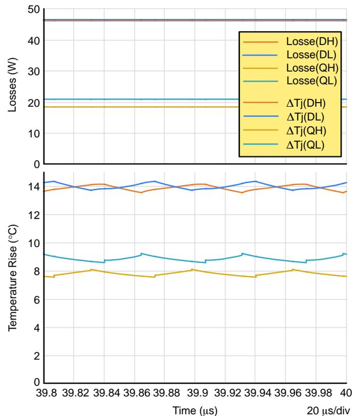
**Figure 33. Losses Measurement Using "TCase" Pin Current/Power Flow and Junction Temperature Rise**
