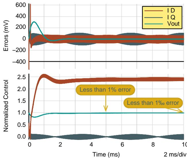
**Figure 40. Control variables and Error Variables. Control and Error Are Not Affected by 3<sup>rd</sup> Harmonic**
