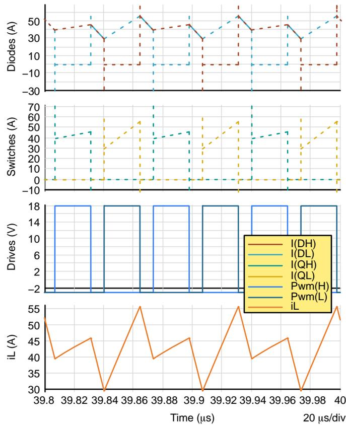
**Figure 29. Flying Capacitor Boost Switches Current Waveforms**
