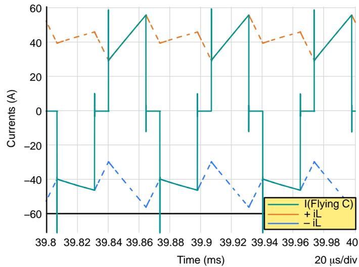
**Figure 30. Flying Capacitor Boost Capacitor Current Waveform**
