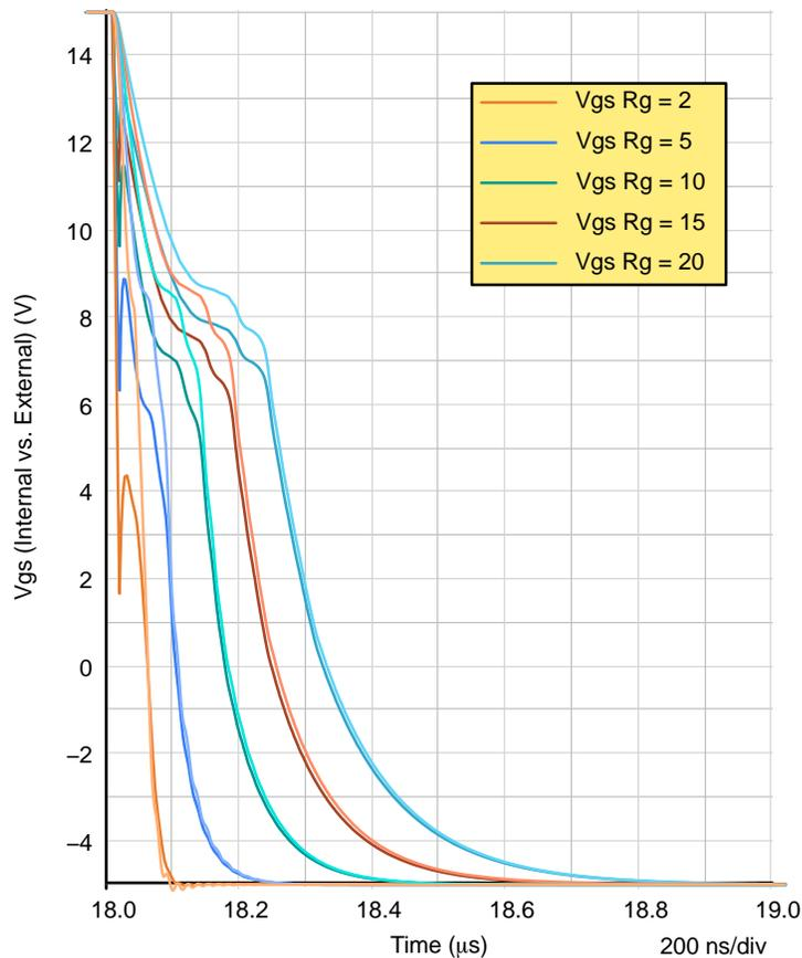
**Figure 8. Gate-to-Source Voltage Difference between Internal and External as a Function of the External Gate Resistor**
