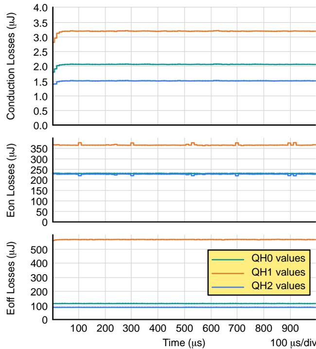
**Figure 17. Turn-On, Turn-Off, and Conduction Losses Energies in Each SiC MOSFET**
