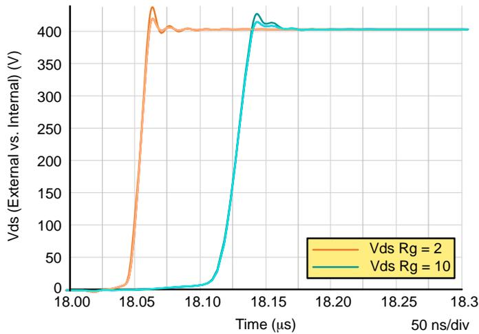
**Figure 7. Drain-to-Source Voltage Difference at Turn-Off between Internal and External**
