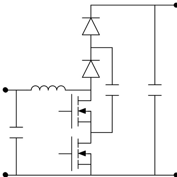
**Figure 28. Flying Capacitor Boost Schematic**
