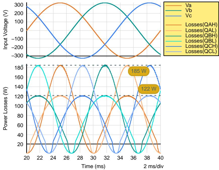
**Figure 43. Losses without Third Harmonic Injection Over On Grid Period**
