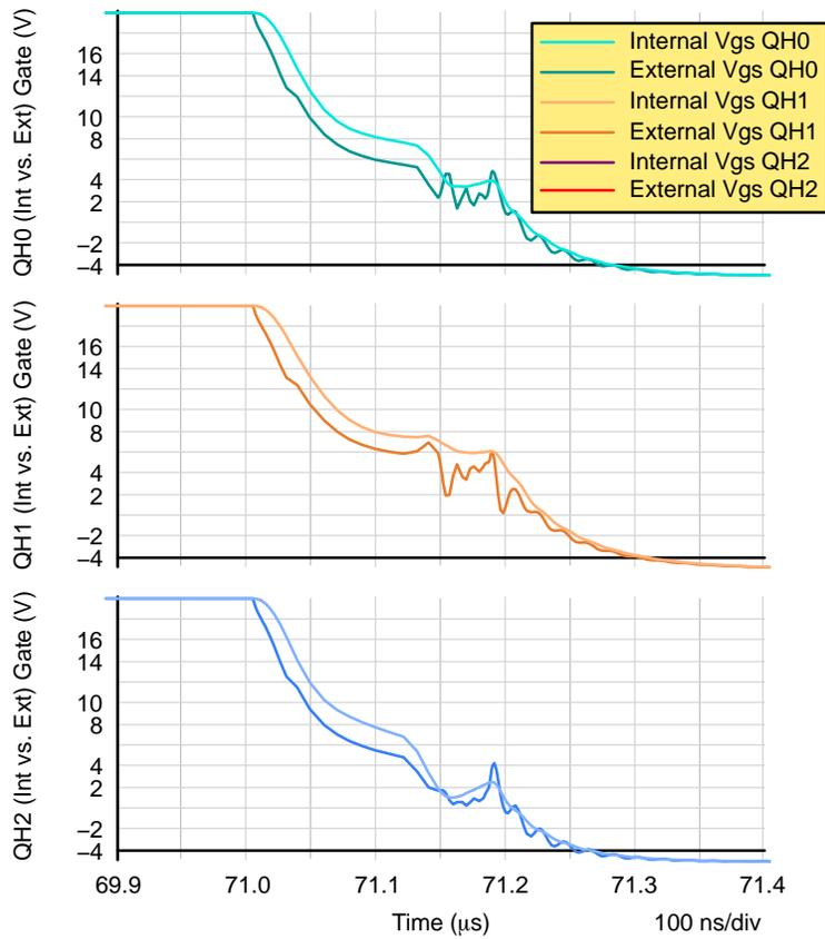
**Figure 15. Turn-Off Sequence Zoom Internal vs. External Gate-to-Source Voltage**
