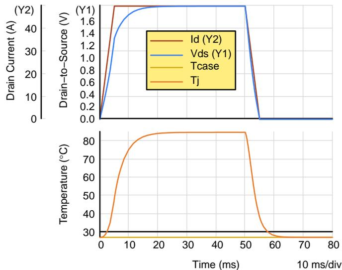
**Figure 20. Junction-to-Case Temperature Difference**
