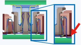
No stress is applied to the leads on the PCB.
