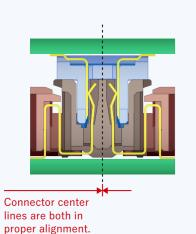
are not perfectly aligned with each other. Movable Portion Joint moves along with the mating connector Alignment Error Springs : Controls Movement
